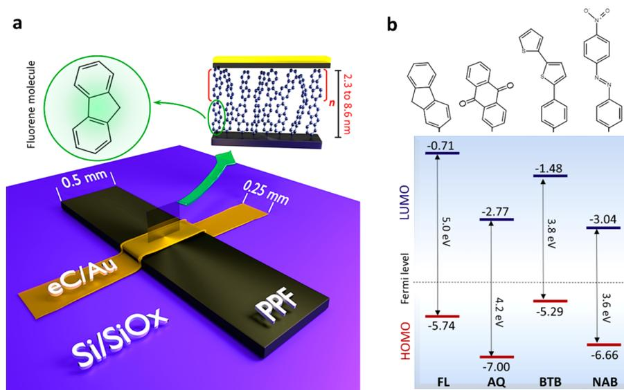
**Figure 1.** (a) Schematic illustration of PPF/FL/eC<sub>10</sub>/Au<sub>20</sub> molecular junction;  $n$  is a number of repeating units of oligomer that determines final thickness of molecular layer. (b) Structures and frontier orbital energy diagram for FL, AQ, NAB, and BTB, relative to a vacuum reference. Orbital energies were calculated by DFT B3LYP 6-31G(d), in Gaussian 09. Fermi level of PPF and eC is  $-4.8$  V vs vacuum.
