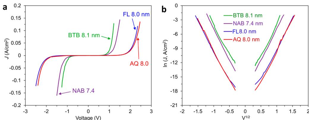
**Figure 6.** (a)  $JV$  curves of BTB, NAB, FL, and AQ with thicknesses close to 8 nm. (b)  $\ln |J|$  vs  $V^{1/2}$  plots for curves in panel a.
