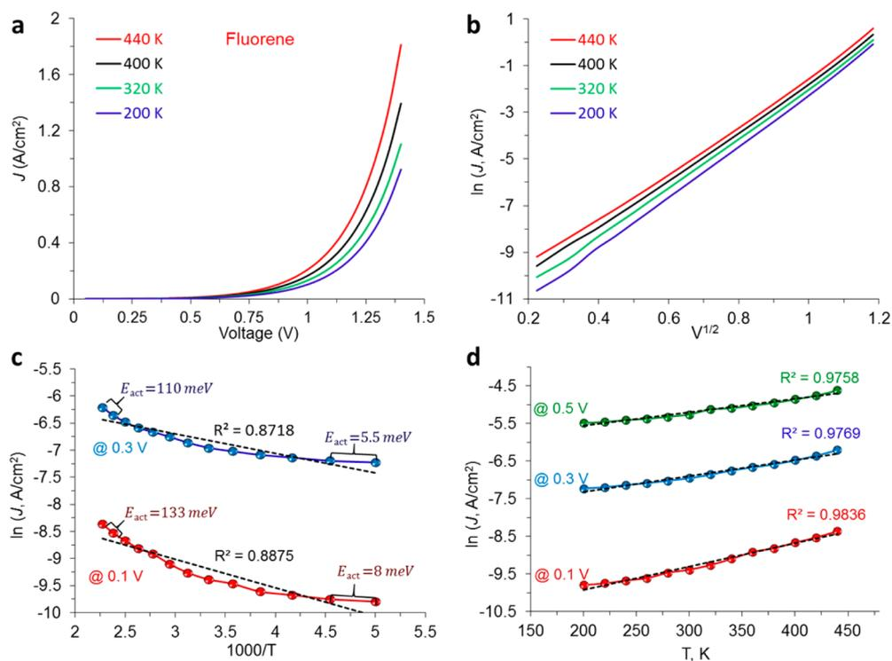
**Figure 4.** (a)  $JV$  curves for PPF/FL<sub>5.5</sub>/eC<sub>10</sub>/Au<sub>20</sub> junction at four temperatures from 200 to 440 K in vacuum. (b)  $\ln J$  vs  $V^{1/2}$  plots for curves in panel a. (c) Arrhenius plots at 0.1 and 0.3 V, with apparent activation energies for high and low  $T$  segments. (d)  $\ln J$  vs  $T$  at 0.1, 0.3, and 0.5 V.  $R^2$  for linear fits of the lines are indicated.
